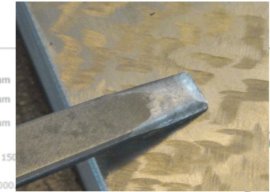
Hand scrapping in all contact surfaces
