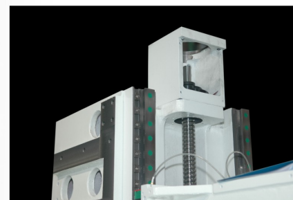
2 linear guide way with 4 slide block in Z axis
