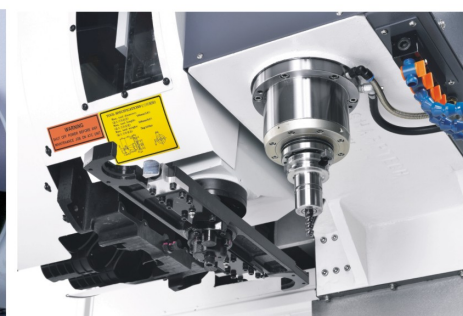
Swing arm ATC and spindle nose
